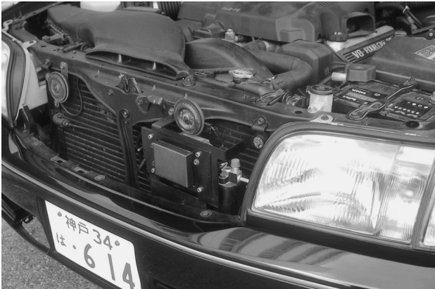
Fig.16 Millimeter-wave radar attachment
