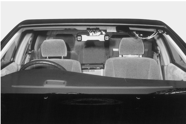
Fig.17 Attachment of image recognition sensor
