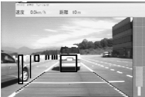
Fig.14 Recognition results 1 (vehicle cut-in)
