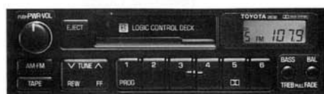
Microprocessor-controlled stereo cassette-deck with AM/FM electronic tuning radio and 4-channel amplifiers
