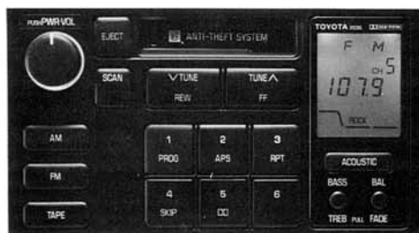
Microprocessor-controlled stereo cassette-deck with AM/FM electronic tuning radio and 4-channel amplifiers having fixed equalizer for acoustic facilities
