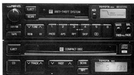
Microprocessor-controlled stereo cassette-deck and CD player with AM/FM electronic tuning radio
