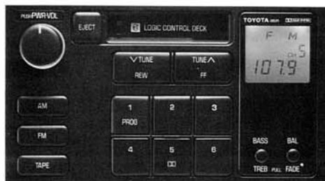
Microprocessor-controlled stereo cassette-deck with AM/FM electronic tuning radio and 4-channel amplifiers
