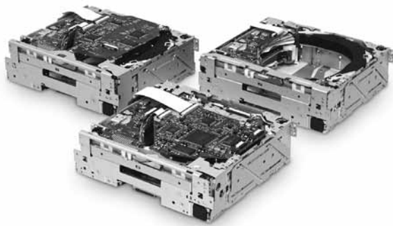
(Front: DVD type, back left: 6 CDs and top print board type, back right: 6 CDs and side print board type)
