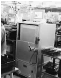
Fig.24 Automatic noise inspection equipment introduced in an actual production line
