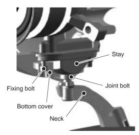
Fig.8 Angle Adjustment Mechanism
