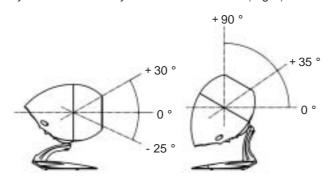
Fig.9 Shift in Angle Adjustment Range by the Assembly Direction of Neck
