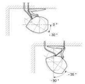
Fig.11 Variations of Installation on a Ceiling
