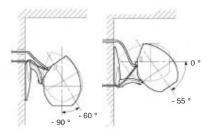
Fig.10 Variations of Installation on a Wall
