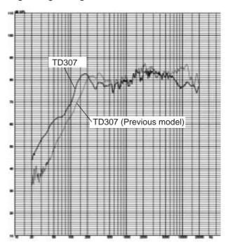
Fig.7 Comparison of Frequency Response
