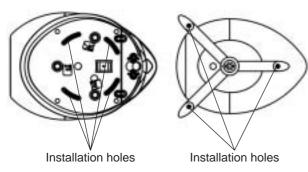
Fig.15 Installation Holes of TD307 and TD307(Previous Model)
