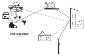
Fig.1 Multipath propagation
