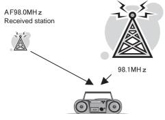
Fig.5 AF check with offset
