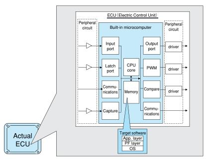
Fig.1 Structure of Real ECU
