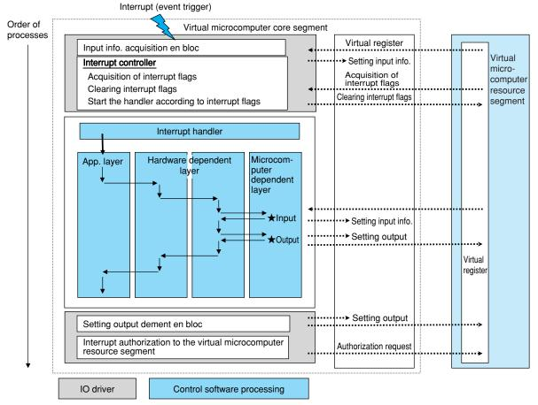
Fig.6 IO Processes on Virtual Microcomputer Periphery
