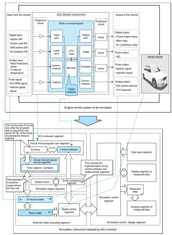
Fig.5 Structure of SILS Type 2 Corresponding to Real Engine Control System
