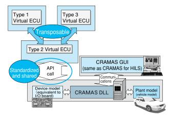
Fig.3 Basic Structure of SILS
