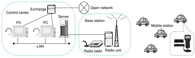
Fig.2 Image Drawing of AVM System Components
