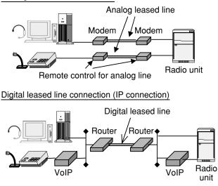
Fig.8 Analog Connection and IP Connection
