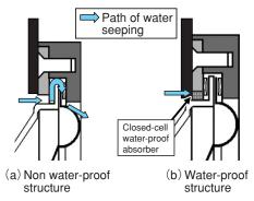
Fig.10 Water-Proof Countermeasure of TD Structure Part
