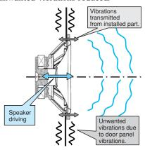
Fig.6 Door Panel Condition with Driving Conventional Custom-Fit Speaker
