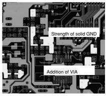
Fig.10 Example of Pattern Reflection
