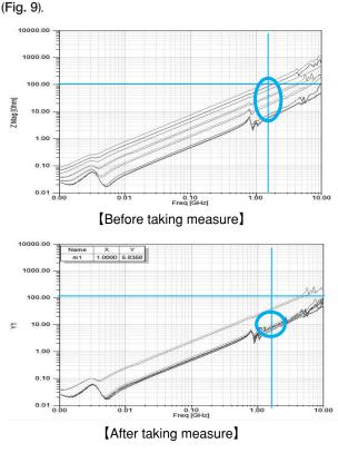
Fig.9 Power Source Impedance
