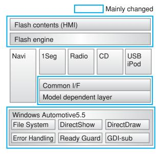
Fig.18 Software Configuration and Main Changed Points
