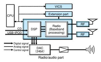
Fig.8 Block Configuration of Radio/Audio
