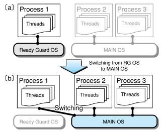
Fig.21 Structure of High-speed Start-up
