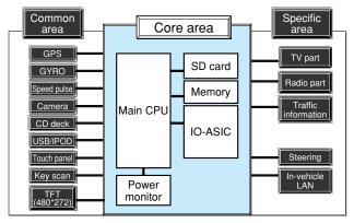
Fig.4 System Configuration Diagram
