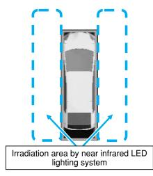
Fig.11 Irradiation Area by Near Infrared LED Lighting of This System
