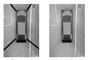
Conventional Multi Angle Vision™ Fig.9 Examples of Borderlines between Camera Images
