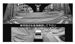
Fig.4 Image Used for Check at Intersection with Poor Visibility
