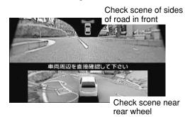
Fig.14 Images Used for Turning Left at Intersection with Poor Visibility
