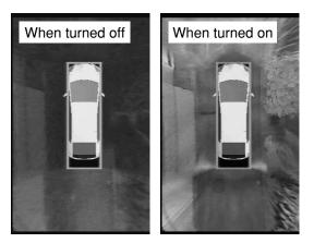
Fig.12 Difference in Brightness of Bird's Eye View Images between with Lights on and with Lights off
