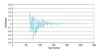
Fig.12 Impulse Response in Targeted Sound Field
