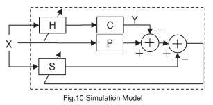
A white noise was used as an acoustic signal (X) in order to assure the precise target sound field.
