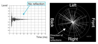
Fig.3 Impulse Response (Left) and Directional Diffusion Diagram of Reflected Sounds (Right) in Vehicle Cabin [with Spatial Control off]
