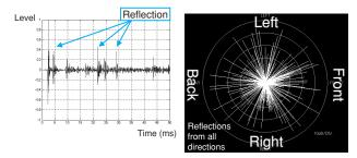
Fig.2 Impulse Response (Left) and Directional Diffusion Diagram of Reflected Sounds (Right) in [Ideal] Living Room
