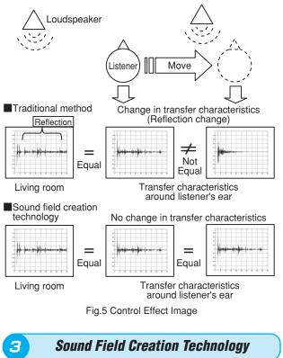
To deal with the tasks, we took an adaptive control technology to control the unnecessary reflection sounds depending on the listener's move. A simultaneous equation method is specifically adaptive to the listener's move among the adaptive control technologies. This method keeps detecting the listener's move and controls the unnecessary reflection sounds depending on the move.
