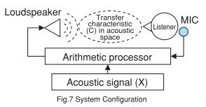
Here, the processing inside the arithmetic processor is described.
