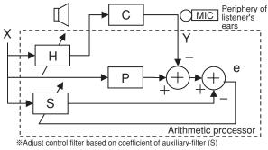
Fig.9 Block Diagram of Arithmetic Processor
