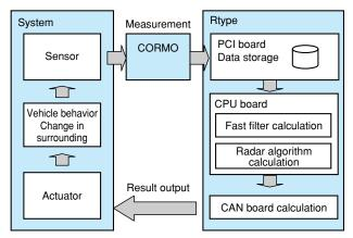
Fig.9 CORMO and Rtype Configuration Diagram
