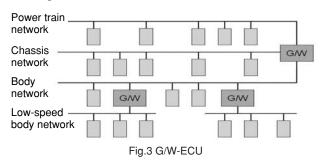
A G/W-ECU is tested in the following points; communication load and condition (sleep/wake-up) of each network, and behavior influenced by bus disconnection/ short-circuit. As for a multi channel type of G/W-ECU, the number of combinations of these tests is larger. To carry out these tests effectively, we have developed the following functions.
