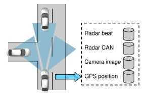
Fig.5 Measurement Data for Millimeter-Wave Radar
