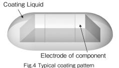
However, condensation forms if even a part of the electrodes of the chip is uncovered (or with no coating material), and the condensation causes the migration. Thus, the entire chip has to be firmly covered by coating material. The film made of dried coating material has to be thick enough not to be ruptured to prevent the migration from occurring at the ruptured part.
