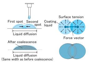
Fig.13 Liquid diffusion by multi-point coating
