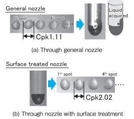
Fig.10 Coating through nozzle
