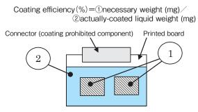
Fig.6 Concept of coating efficiency
