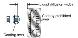
Fig.9 Target width of liquid diffusion
