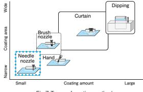
Fig.7 Types of coating method
