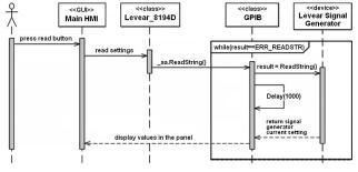
Fig.4.2 Sequence for reading signal generator settings
