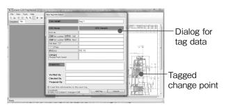
Fig.3.4 Setting screen for drawing output of comparison result
