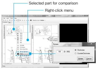
Fig.4.4 Rotation angle correction
