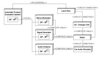
Fig.2.1 APES system configuration
