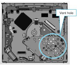
Fig.7 Heat Release Hole of Deck Chassis
