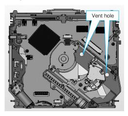
Fig.8 Heat Release Hole of Pickup Chassis
