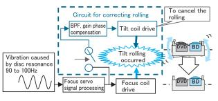
Fig.10 Block Diagram of Rolling Correction Circuit
