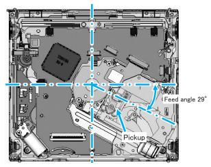
Fig.3 Pickup Layout on DV-05
