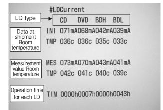
Fig.14 Sample Display of Diagnosis Result regarding Laser Current Value
