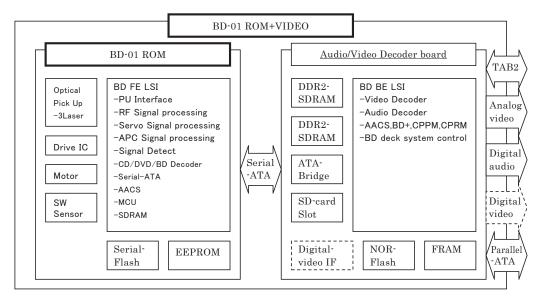
Fig.5 System Block Diagram
