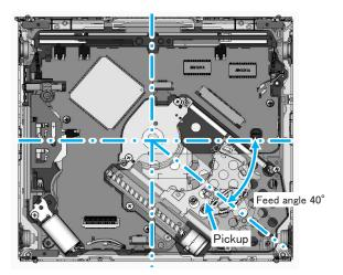
Fig.4 Pickup Layout on BD-01
