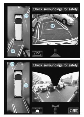
Fig.2 Screens Showing Guiding Lines for Parking
