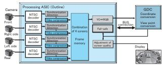
Fig.7 Block Diagram of Image Processing ASIC and Its Peripherals
