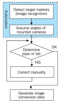
Fig.9 Flowchart of Calibration
