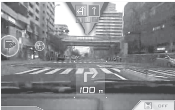
Fig.4 Example of screen display of AR navigation system using WebRTC and Canvas
